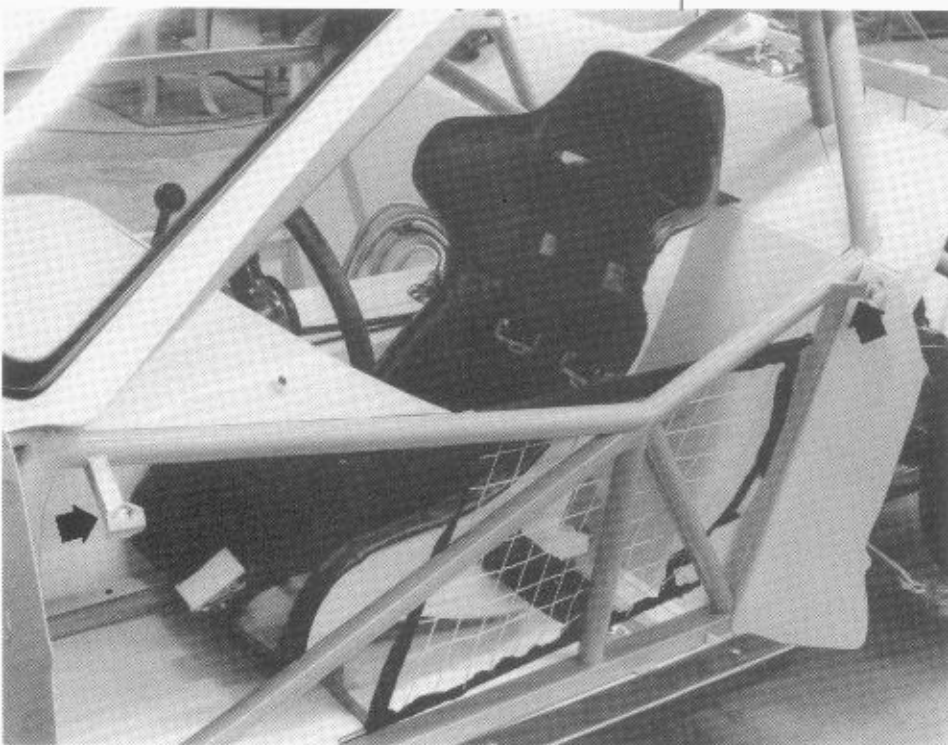
ABOVE—This view shows how the coolant transfer lines are routed into the engine bay and around the suspension components. Flexible connections are made at this point, but they have to pass over and under the right rear radius rods without interference.
