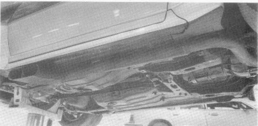
The exhaust system features a single competition muffler with 3-inch-diameter tubing from the header to the expanded dual outlet. The bottom of the car doesn't look altered at first glance, but a closer inspection will show that all body seams in the unibody structure have been welded to increase the structural integrity of the chassis.
