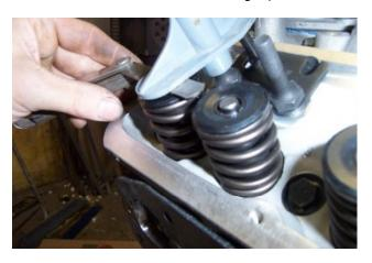
The picture shows the Manley pushrod length checker for small-block Chevy engines. The engine here has a cam with 0.510" lift. In order to get the proper length, I need to subtract 0.510 from 0.600 to get 0.090". 0.090 divided by 3 is 0.030.
