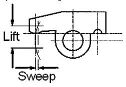
Proper geometry is very important to limit guide wear. Another plus of making rockers with the pivot point on a lower plane than the pushrod cup and valve tip contact point is that the maximum rocker ratio will not be the same point as minimum movement. That will allow us to get some more power; I'll discuss that in the Optimizing Geometry section.
