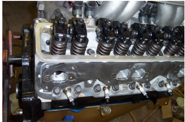
This is what the adapter flanges look like when port matched to the heads. It's hard to see in this picture, but some of the bolt heads need to be ground off. This is normal for large ports.
