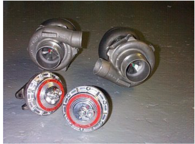
Here are the turbochargers & waste gates as I go them from Turbonetics. These are with the original 0.69 A/R housings.
