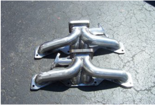
These are the completed headers with the welds ground smooth ready to be sent to Jet Hot for coating.
