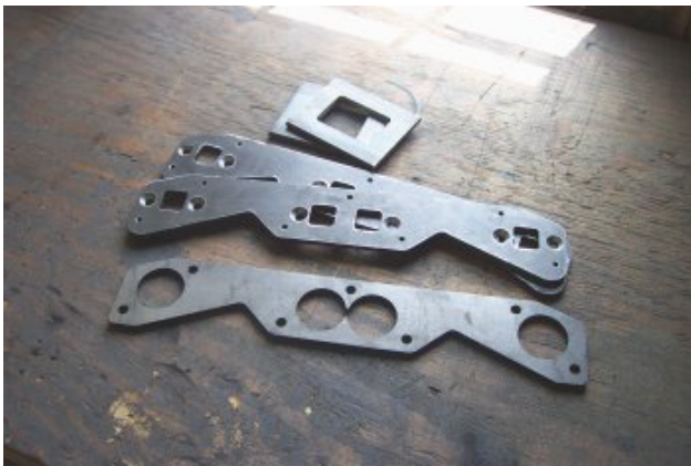
Here's the flanges needed to use big tube headers with a small-block Chevy pattern.
