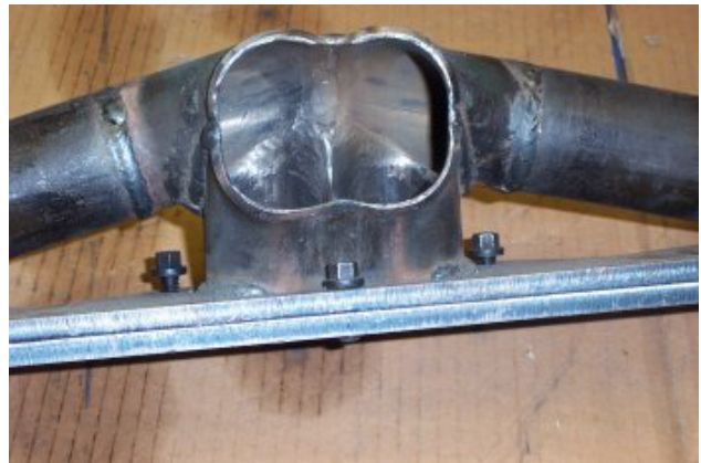
Here's a look down the collector before the turbo flanges and waste gate piping was welded on.
