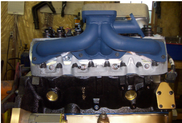
Here is the headers coated & installed on the engine.
