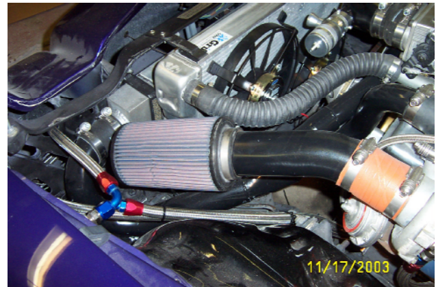
With the radiator moved back, the intercooler fit in with little problem.
