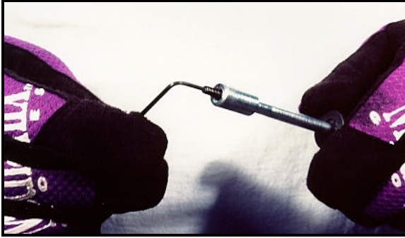
When flap wheel work is done, an Allen stud goes in its place.
