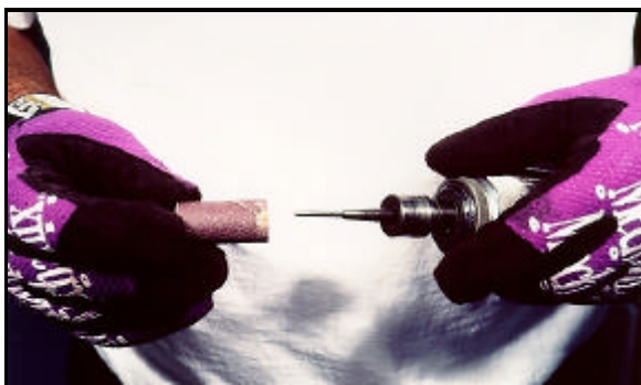
The cartridge roll mandrel has threads that hold the roll. Each roll has an orange spot which is pointed at the grinder. All you do is push the cartridge roll on the mandrel, then screw it tight.
