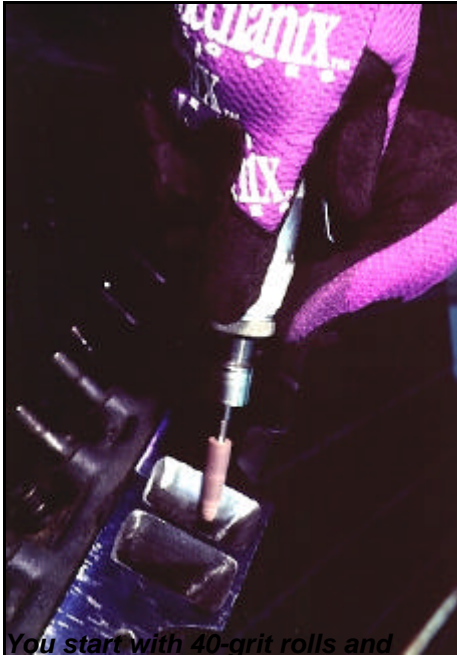
You start with 40-grit rolls and progress to 80-grit. In many intake ports, the small-diameter rolls will be needed to finish the radii at the corners of the port. Typically you polish only 1-1.5 inches down the port.
