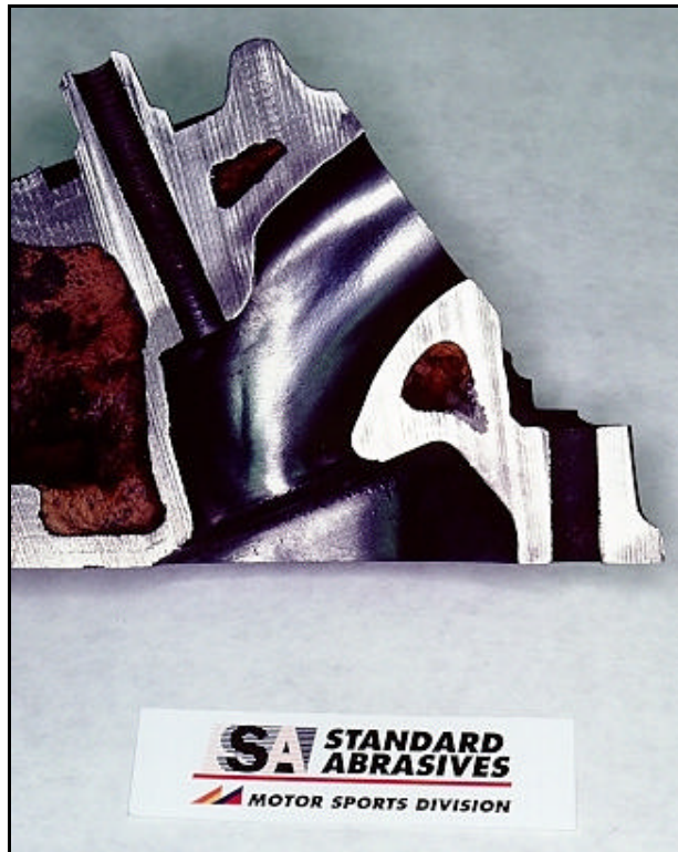
This is a finished exhaust port. Not the smoothed valve guide and short side radius. Also, note the finish is significantly different from what we saw on the intake cutaway.
