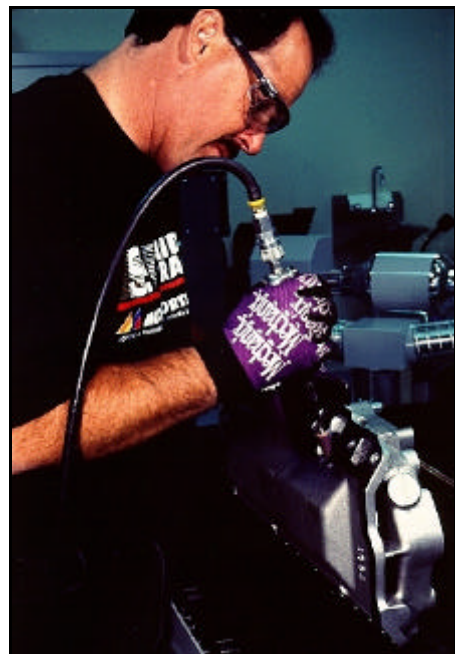
The Fel-Pro intake gasket is used again to mark the manifold. You want the top of the gasket to face the manifold whereas you had the bottom of the gasket facing the head.
