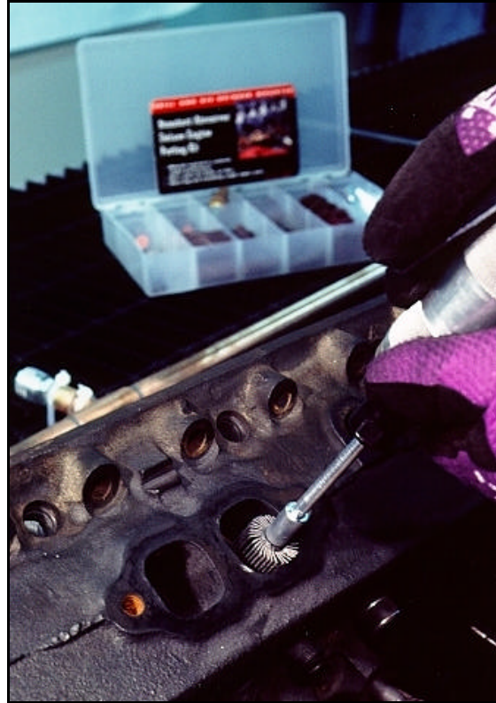
You want to flap wheel all accessible areas of the exhaust port.
