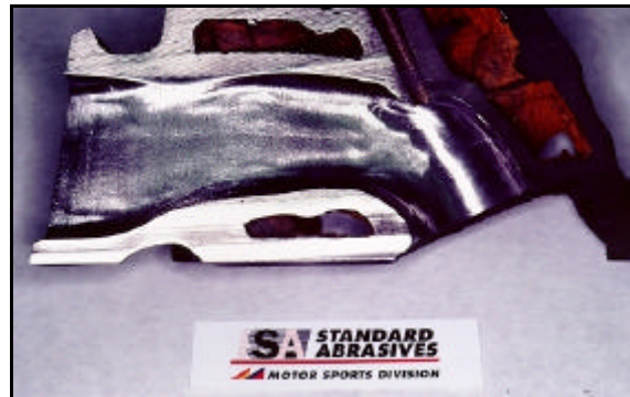
With this cutaway, we polished the whole port to better illustrate the rough-to-touch finish. Note the smoothed valve guides and short side radius.
