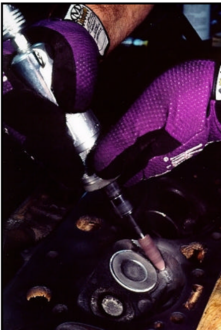
Half-tapered cartridge rolls are best to polish chamber corners.
