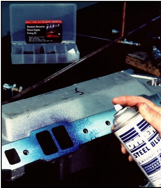
The spray Dykem is again used on the intake manifold.
