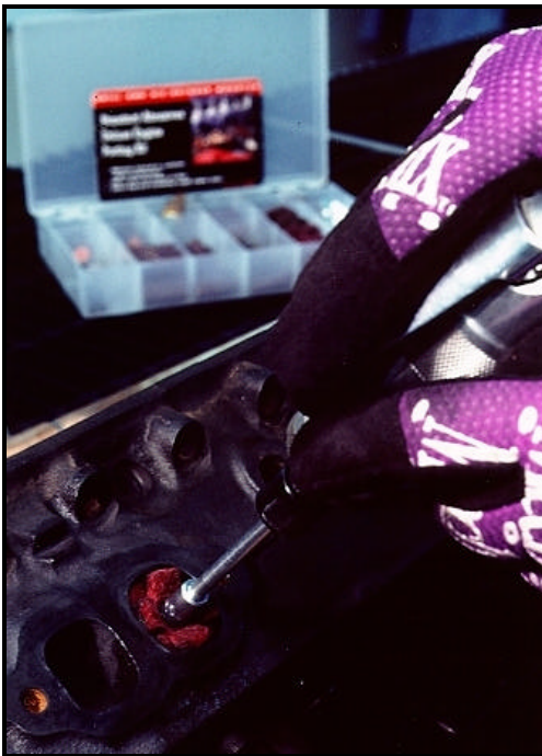
When flap wheel work is done, an Allen stud goes in its place.
