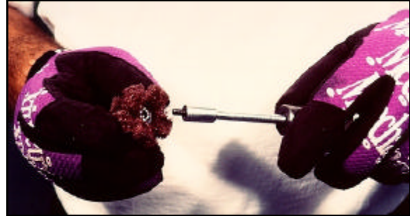
Cross Buffs™ are screwed onto the Allen stud in the Combination Mandrel.
