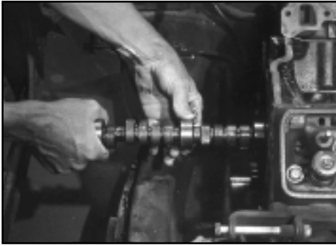
Figure 4. Be sure not to wipe away any of the assembly lube as you install the cam into the block. Some motor oil on each cam bearing journal also helps make this step easier.
