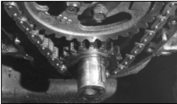
Figure 5. Timing marks must be exactly lined up. Our small block Chevy has a "dot over dot" arrangement, as shown. Consult your shop manual for exact arrangement of your engine.
