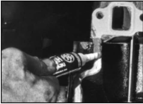
Figure 12. A silicon sealant (fast curing) should be used on end-rails as shown. This prevents annoying oil leaks. Do it right the first time and forget it!
