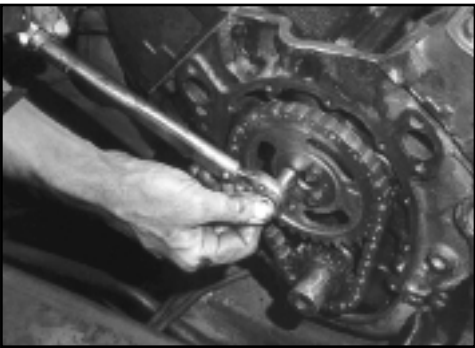
Figure 6. When the timing marks have been correctly aligned (check and re-check this before proceeding!) you can re-install the cam sprocket bolts. Use a vibration-dampening adhesive, such as Loctite compound. Torque each bolt to factory specs.
