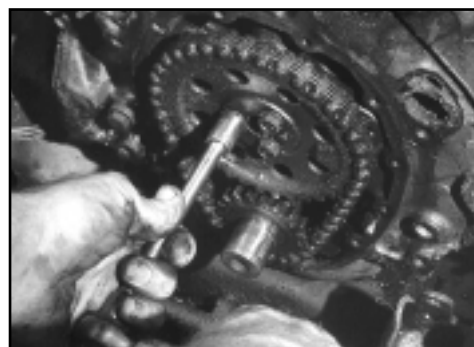
Figure 2. Loosen cam sprocket bolts and remove them. Place in a container and label or tag for later re-use.
