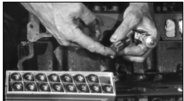
Figure 8. Apply a generous amount of assembly lube to each lifter bottom.
